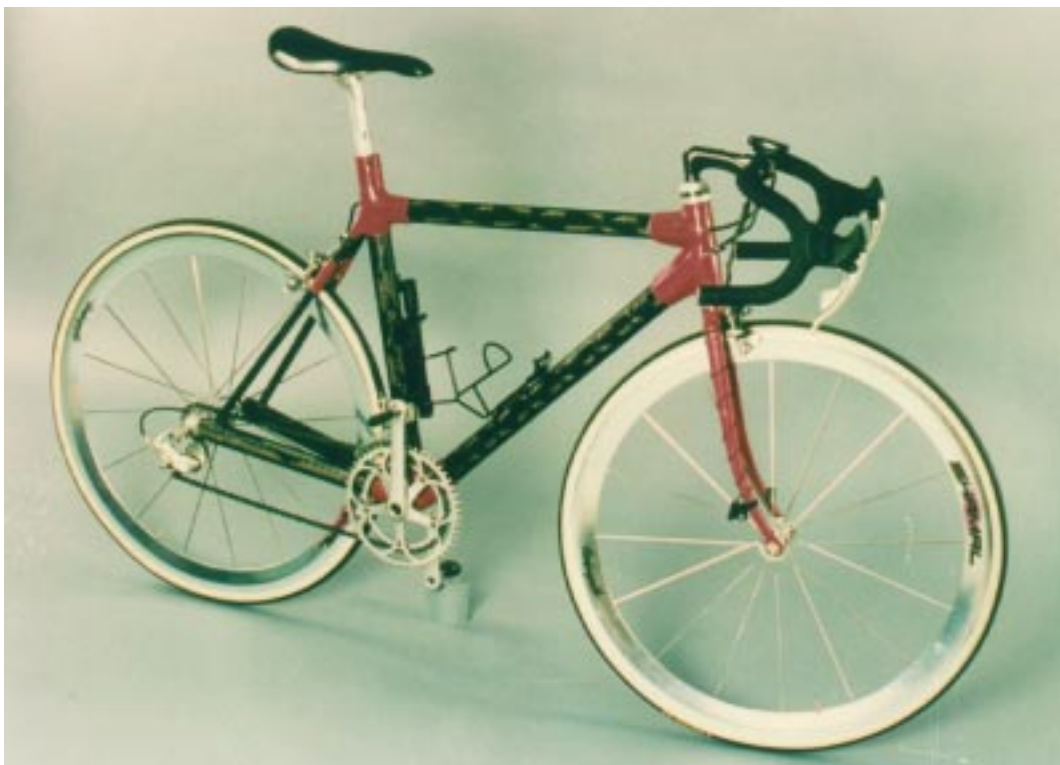
Fig. 3: Thermoplastic filament wound bicycle frame
