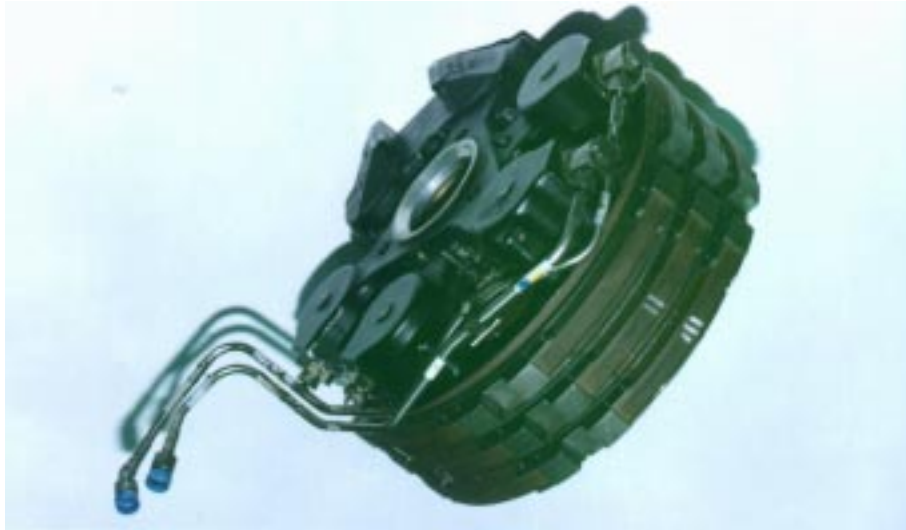
Figure 1: Photograph of the prototype brake assembly
