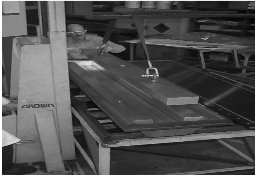
Figure 3: Mandrels in RTM tool.
