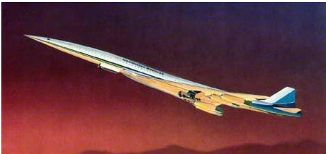
Fig. 2: The proposed Mach 2.4 High-Speed Civil Transport (HSCT) will supersede the Concorde as the next-generation supersonic passenger aircraft
