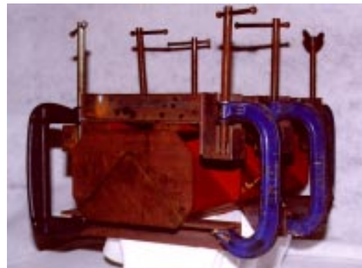
(a) (b) Fig. 2: RTM tool in (a) unassembled form and (b) assembled form.
