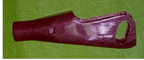
Fig.15 Final Form of Manufactured Artificial Leg Shell
