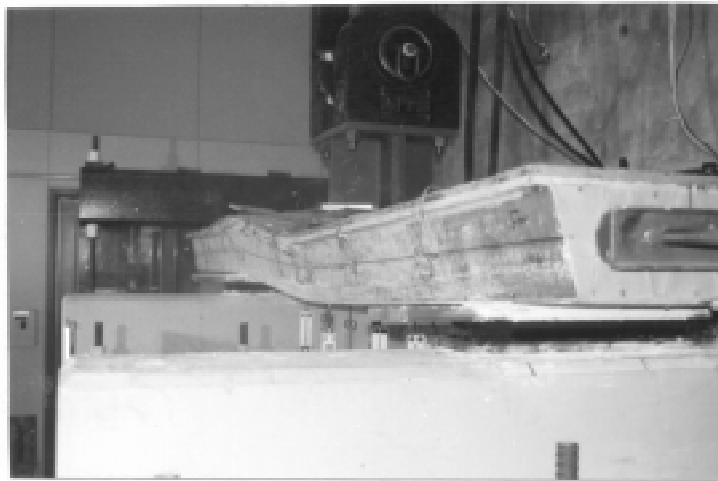
Figure 7b: Deformation of a Trapezoidal Core Component at a Load Level of 215 kips
