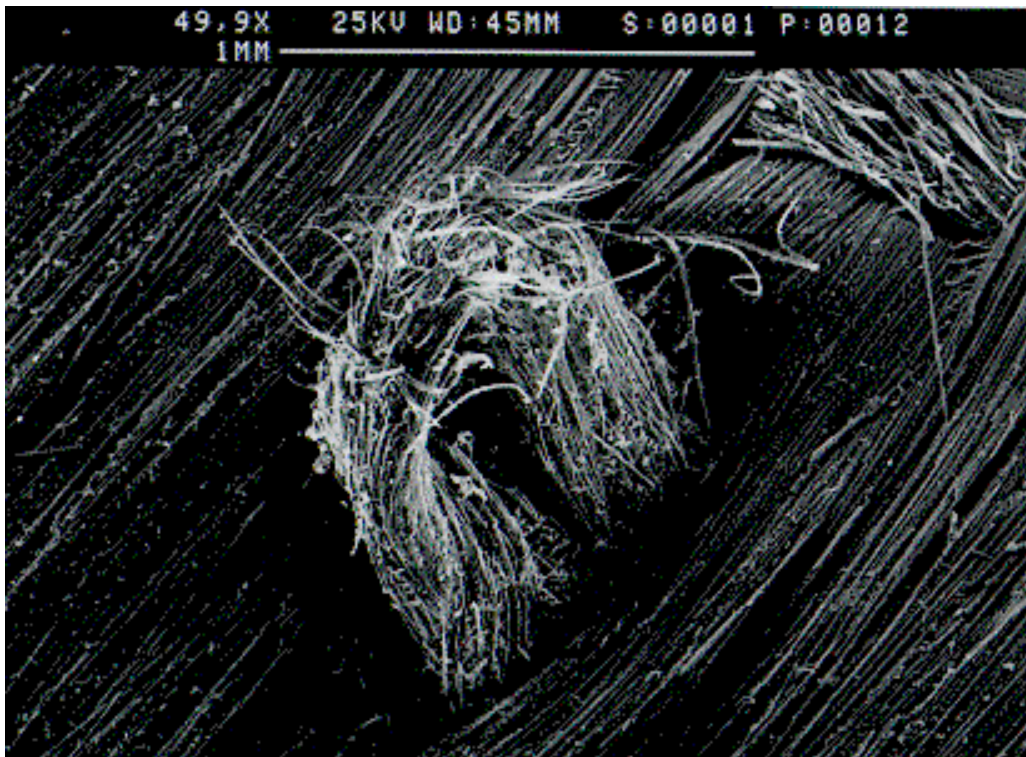
Fig. 8: SEM fractograph displaying thread loop pull-out failure behaviour under mode I loading of a tabbed, Kevlar thread stitched specimen (After [20]).
