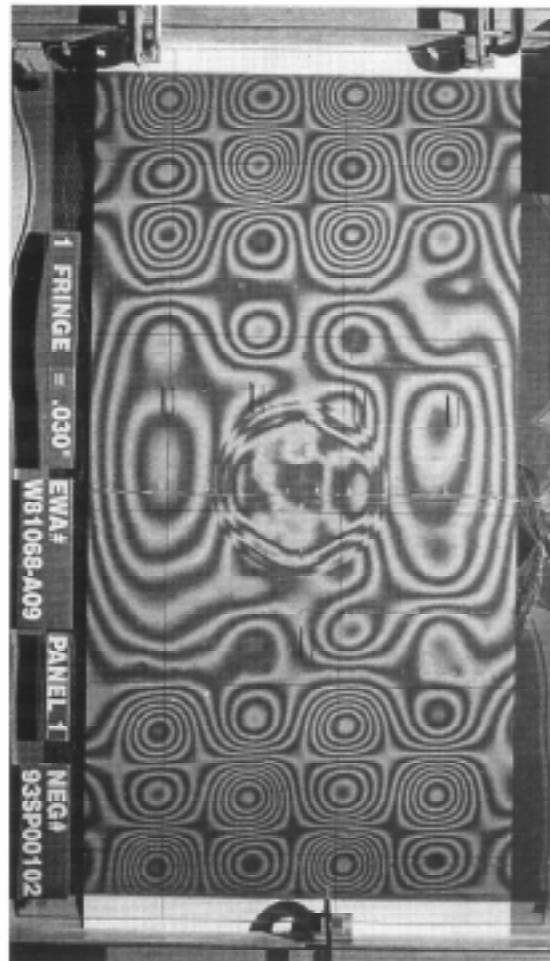
Figure 11: Bonded Repair on CFRP Skin Panel Test
