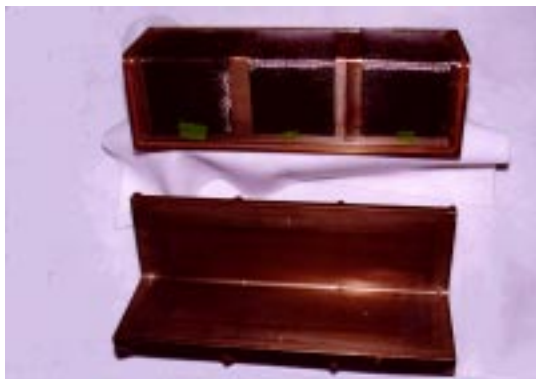
(a) (b) Fig. 2: RTM tool in (a) unassembled form and (b) assembled form.
