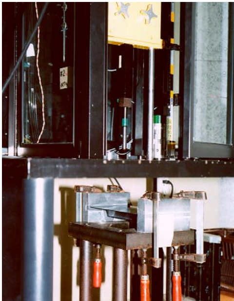
Fig. 3: Photo of impact test by drop weight impactor
