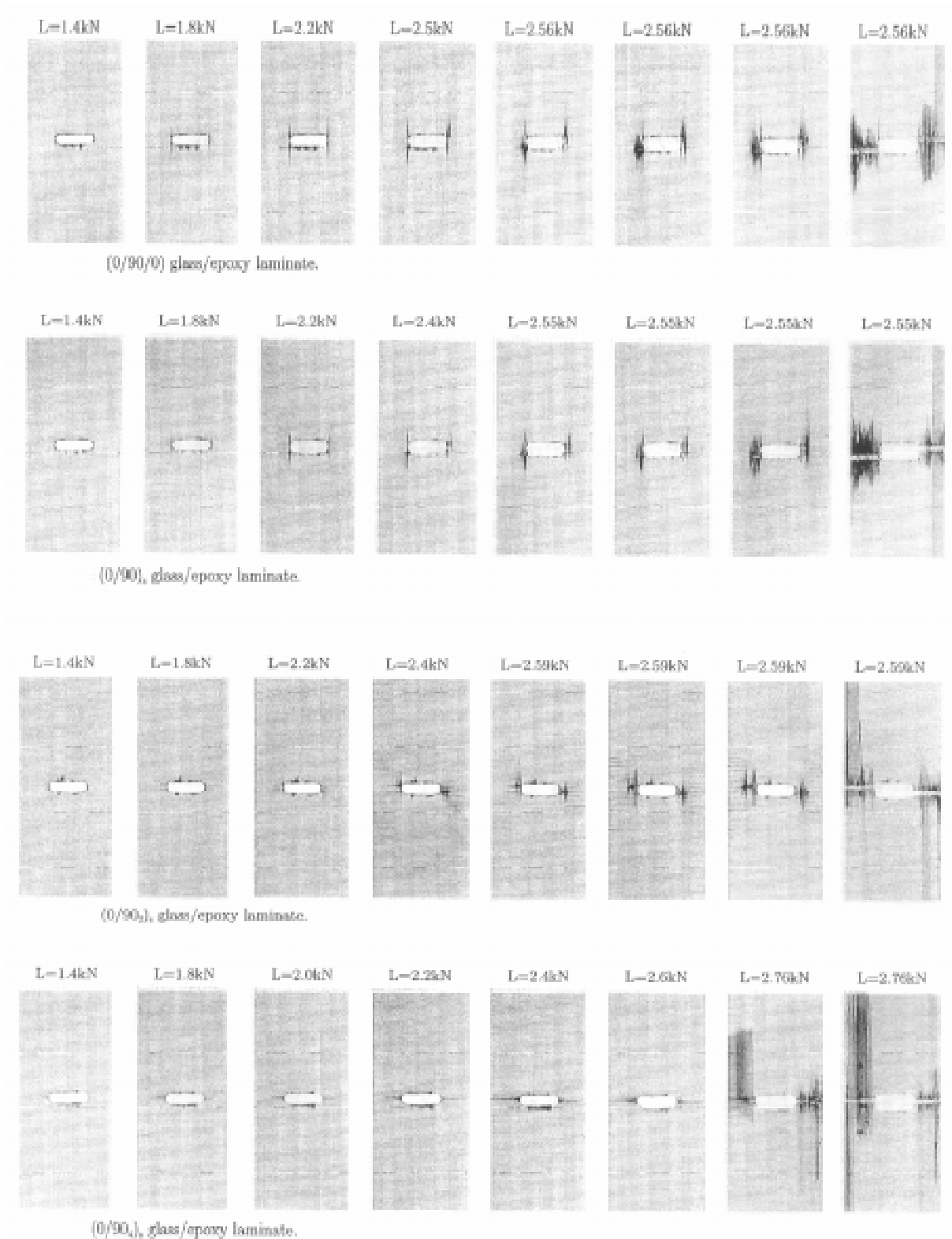
Fig. 1: Sequence of X-ray pictures showing the effects of load and transverse ply thickness on damage growth in glass/epoxy
