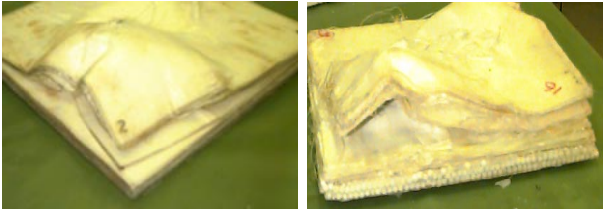
Fig.7: Typical Delamination and Out-of plane deformation of the Spectra Shield® A - Panel No. 2 and B - Panel No. 16
