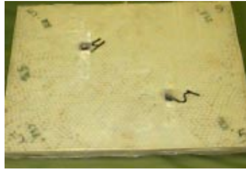
Fig. 6B: Penetration hole panel No. 5 (1 layer)
