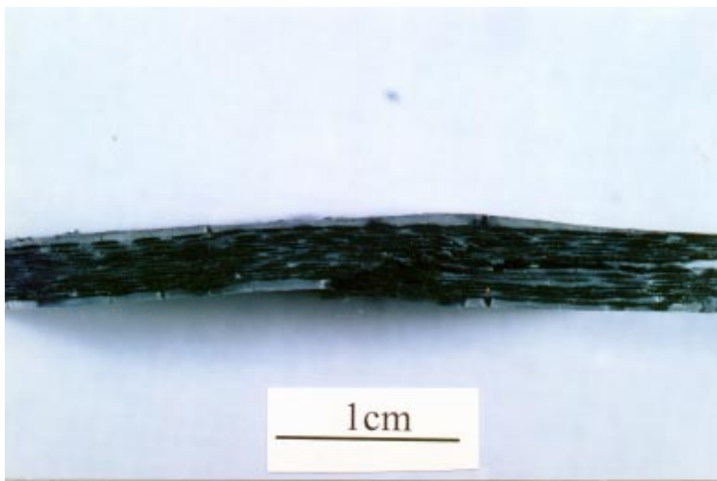
Fig. 5(a): Overview of failure of 2-D carbon/alumina composites showing first major failure mode delamination (fibers treated)
