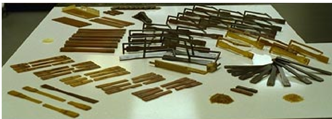
Figure 2: LaRC-SI and LaRC-IAX tensile test specimens
