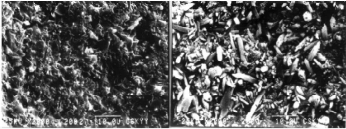
Fig. 3: Microstructure of the etched and fracture surface of sintered parts
