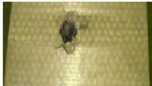
Fig. 6E: Penetration hole panel No. 23 (1/2'')
