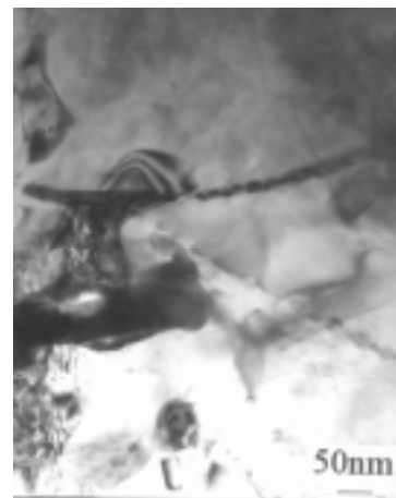
Fig.1: Deforming process of metal powder particles Fig. 2: TEM picture of the interfaces of aluminum powder particles
