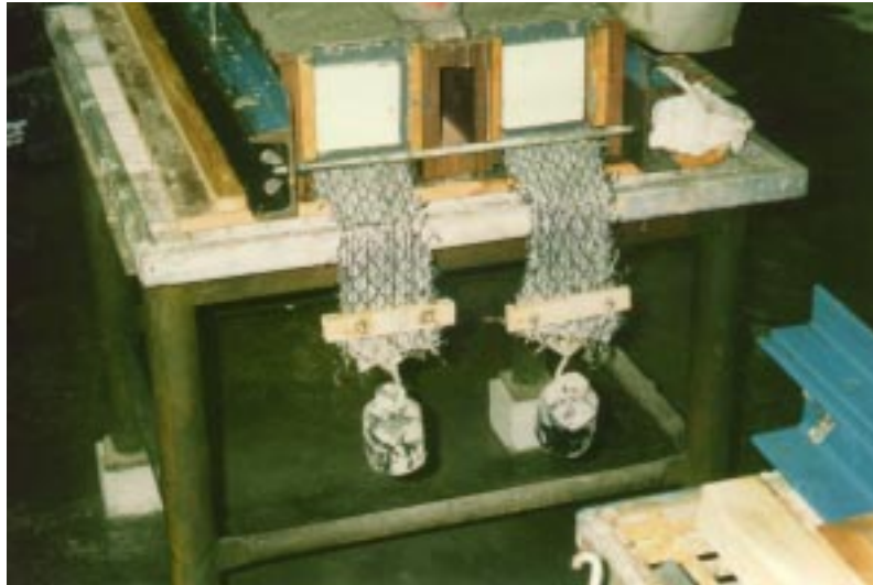
Fig. 7: Production of a Window Lintel
