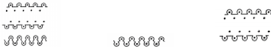
Figure 1: a) Full Milano b) 1x1 Rib, c) plain tubular jersey nomenclature
