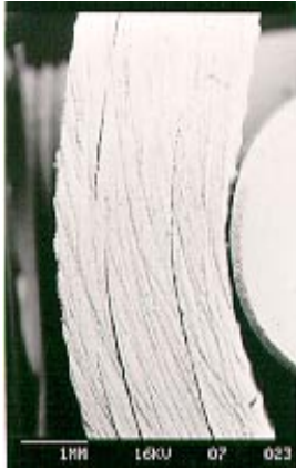
(a) T300/MBMI [0] (b) T300/EP [0] Fig. 7: Interlaminar shear failure at 200°C
