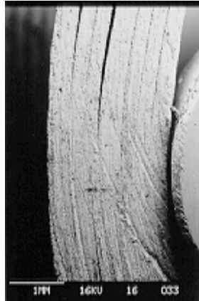
(a) T300/MBMI [0] (b) T300/EP [0] Fig. 7: Interlaminar shear failure at 200°C
