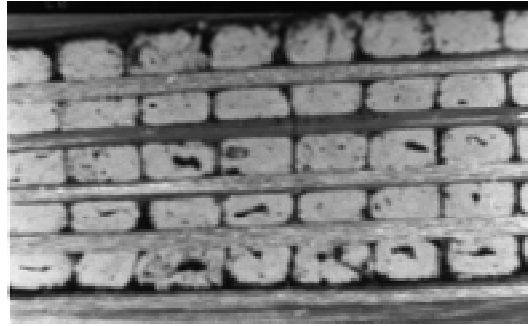
Fig. 4: Multilayer woven structure with a 'near square shape' binder path, consolidated without pressure (sectioned along warp direction)
