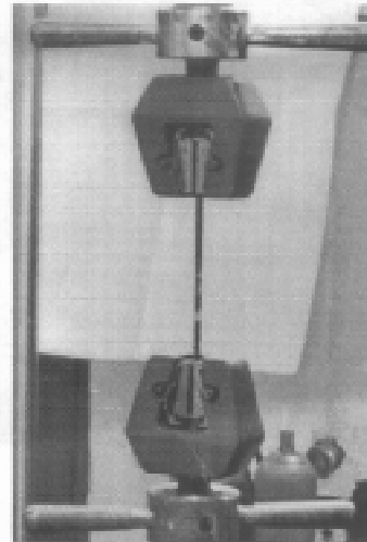
Fig. 3: Overview of the tensile coupon test
