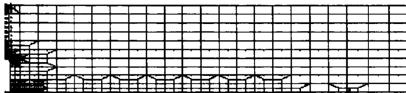
Fig. 13 : Mesh division of the FEM analysis for the specimen.
