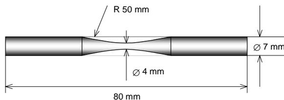
Fig. 1: Schematic of the fatigue test specimen. (cylindrical hour-glass specimen)
