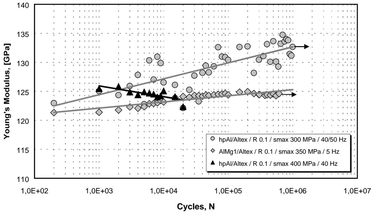
Fig. 9: Variation of the Young's modulus during fatigue life for hpAl/Altex and AlMg1/Altex at 25°C, R 0.1,  $\sigma_{max}$  400 MPa / 40 Hz, 300 MPa / 40-50 Hz, and 350 MPa / 5 Hz respectively. (Note that the specimens tested at R 0.1, 300 & 350 MPa did not fail)
