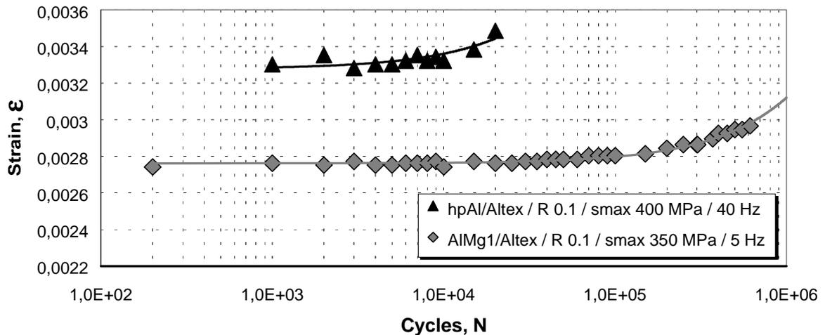
Fig. 10: Variation of the strain during fatigue life for hpAl/Altex and AlMg1/Altex at 25°C, R 0.1,  $\sigma_{max}$  400 MPa / 40 Hz and 350 MPa / 5 Hz respectively.
