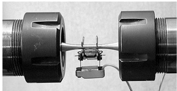
Fig. 2: Test set-up for the stress/strain measurements during cyclic axial loading.
