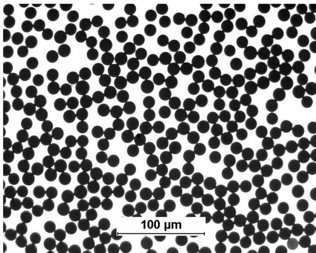
Fig. 3: Typical microstructure of Altex-reinforced Al-based MMCs showing a macroscopically uniform fibre distribution.
