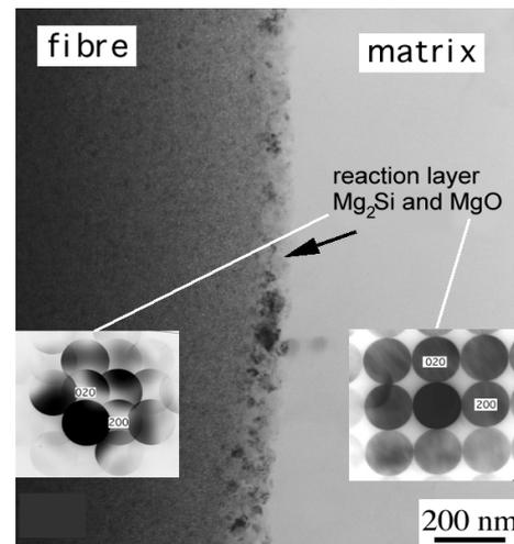
Fig. 4: Interfacial reaction layer in AlMg1/Altex MMCs. (note that hpAl/Altex is free of reaction)
