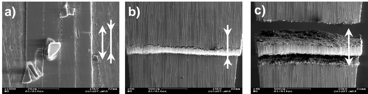
Fig. 12: Failure damage of AlMg1/Altex is initiated by fibre breakage (kinking) (a), followed by matrix shear deformation and subsequent macroscopic kinking (b-c); (R -1, RT).
