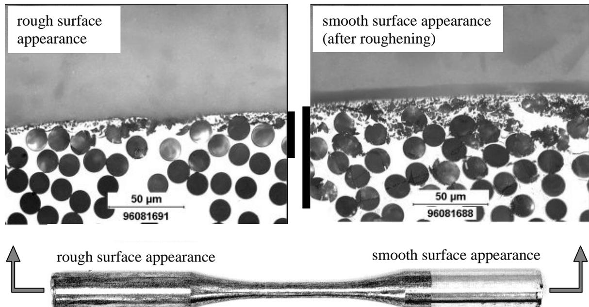
*Fig. 6: Influence of machining conditions on the depth of the damage zone in unidirectional continuous fibre reinforced MMCs: more than 5 fibre layers damage depth after roughening (right), 1-2 fibre layers damage depth after turning with optimised parameters (left). (note that bright fibre reflection signalises in-depth fibre breakage)*
