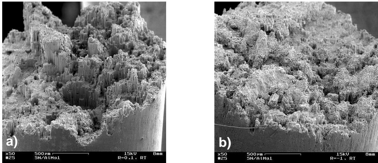
Fig. 13: Fractography of AlMg1Altex at 25°C, R 0.1,  $\sigma_{max}$  400 MPa (a) and at 25°C, R -1,  $\sigma_{max}$  300 MPa (b). Note the contrast between the rough, ductile fracture surface with multiple fibre cracks and protruding fibres (covered by a matrix layer) under pure tensile load in (a) and the flat, crushed fracture surface under reversed loading in (b).
