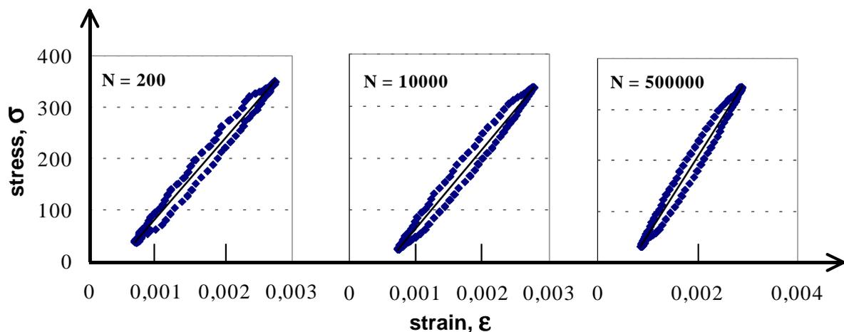
Fig. 8: Typical stress-strain hysteresis loops for AlMg1/Altex at 25°C, R 0.1,  $\sigma_{max}$  350 MPa / 5Hz at different cycle numbers.
