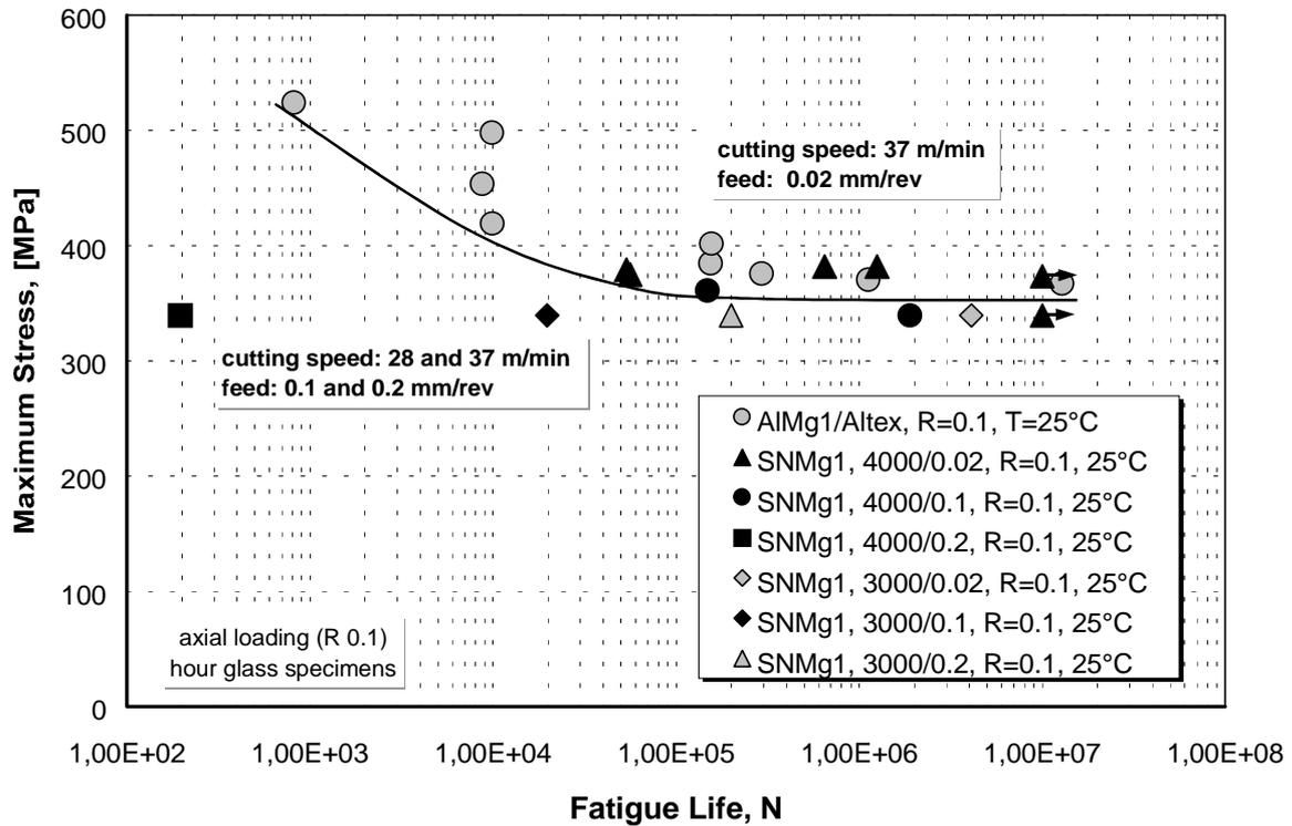
Fig. 7: Influence of the turning parameters on the fatigue endurance of unidirectional continuous Altex fibre reinforced Al-based MMCs. Note the adverse effect of high cutting feed on the composite's fatigue performance. (3000/4000 rpm  $\Rightarrow$  28/37 m/min)
