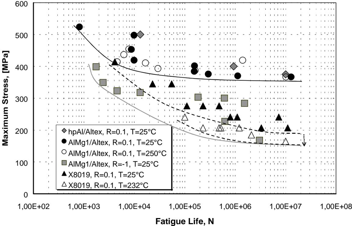
Fig. 5: SN-curves of AlMg1/Altex for various testing conditions compared to hpAl/Altex and an elevated temperature PM AlFe8Ce4 alloy (X8019). Note the insensitiveness of the fatigue performance of AlMg1/Altex to elevated temperatures up to 250°C.
