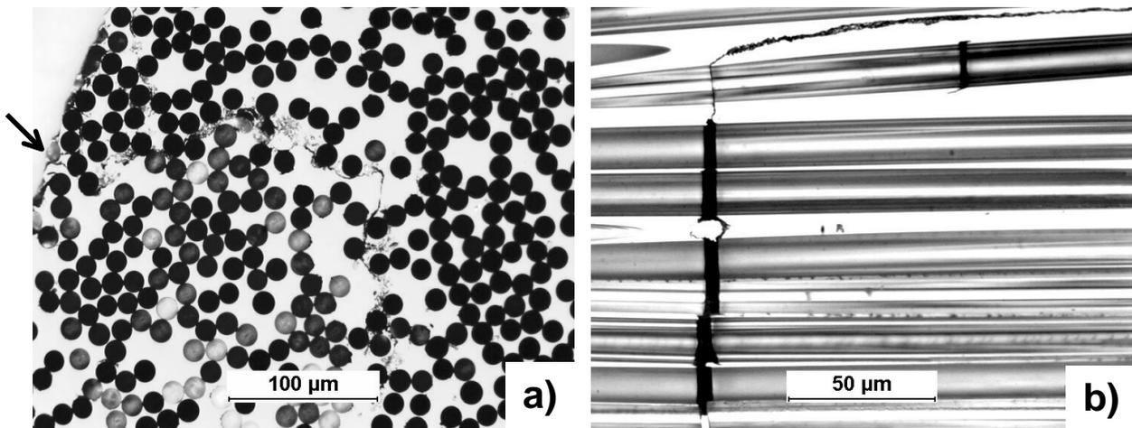
Fig. 11: Development of cracks in the late stages of the fatigue life in hpAl/Altex at 25°C, R 0.1,  $\sigma_{max}$  300 MPa /  $N 10^6$  (a) and  $\sigma_{max}$  400 MPa /  $N 2 \cdot 10^4$  (b). Note the crack initiation at the surface in (a) and the broken fibres (bright reflection) in the area of the crack initiation (the specimen in (a) did **not** fail at  $N 10^6$ ; test was stopped).
