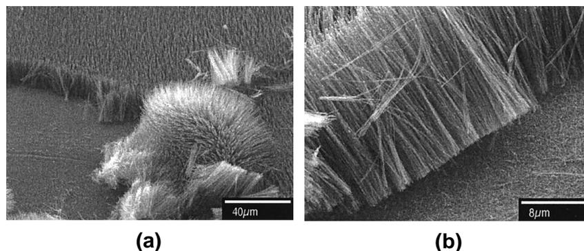
Fig. 3 SEM micrographs showing (a) excellent alignment and uniformity of carbon nanotubes grown over a large area and an enlarged view of the nanotubes along the scratched edge to show uniformity in length, diameter, and site density [15].
