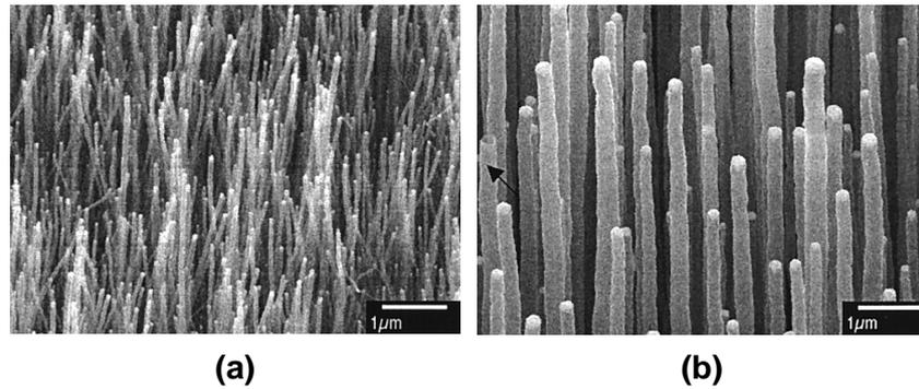
Fig. 4 SEM micrographs showing control over nanotube diameter 40-50 nm (a) and 200-300 nm (b) aligned carbon nanotubes [15].
