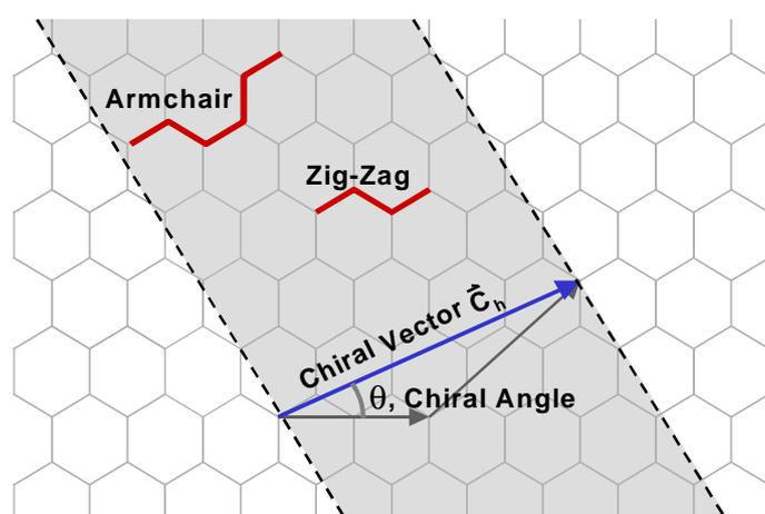
Fig. 1 An illustration of how carbon nanotubes are formed via “rolling” sheets of graphite to form a tube.
