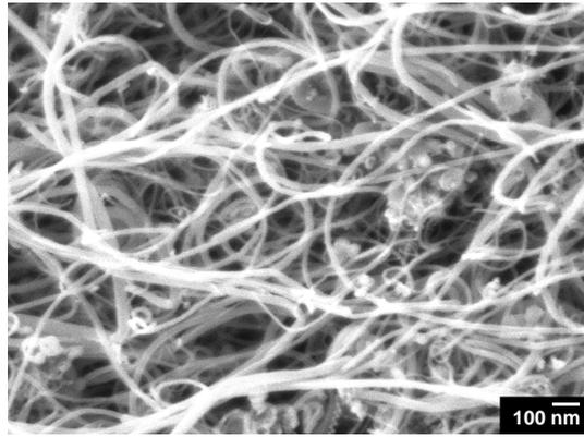
Fig. 6 SEM micrograph showing tangled, spaghetti-like carbon nanotubes grown with conventional CVD techniques [10].
