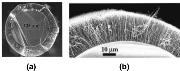
Fig. 5 SEM micrographs showing (a) the radially grown nanotubes on the surface of an optical fiber and (b) a close-up showing the perpendicular nature of nanotube growth [17].
