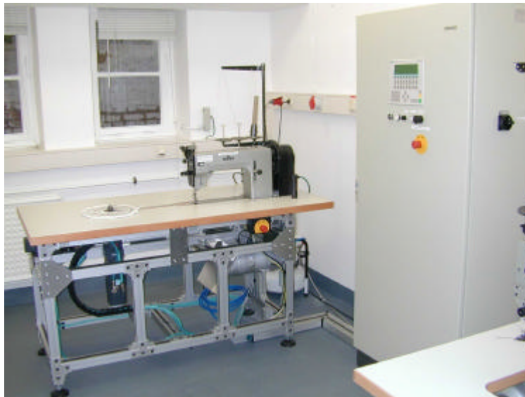
Fig. 7 Sewing unit for pre-fabrication of the rotor disc
