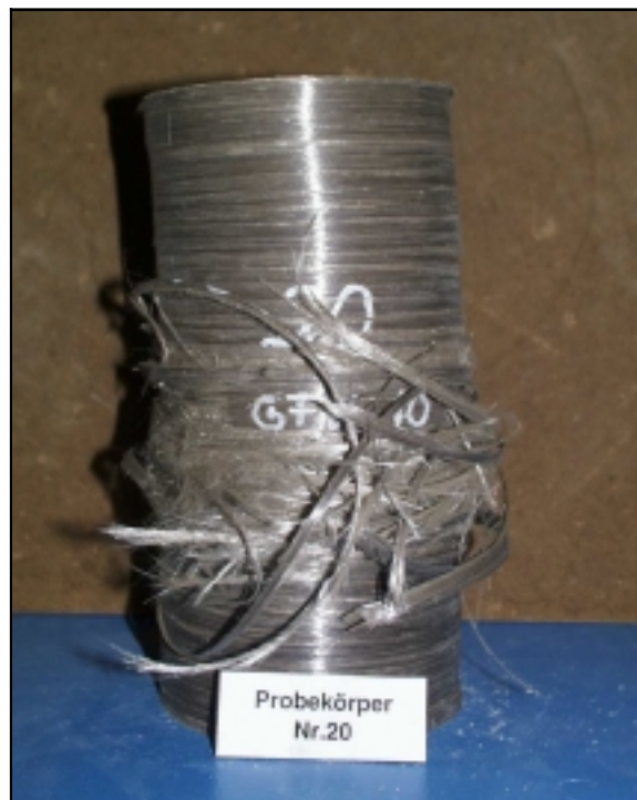
Figure 6: Failure of a GF/PPS shell reinforced concrete specimen
