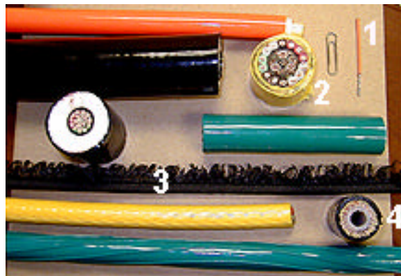
Figure 8 – Collection of Cable Sections, Including the Hair-Fairing and the Buoyant.
