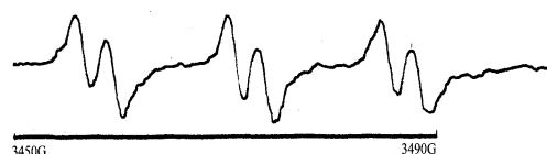
Fig.3 ESR graph of epoxy propane mixture containing 1.5wt% diaryliodonium salts after EB radiation
