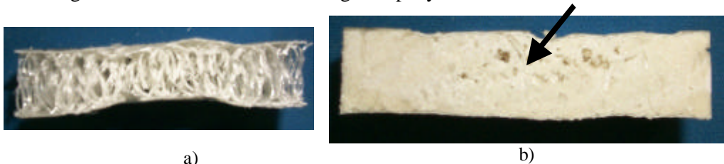
Figure 7. High velocity impact test on integrated core, a) open space, and b) polyurethane foam-filled, arrow represents localized debonding
