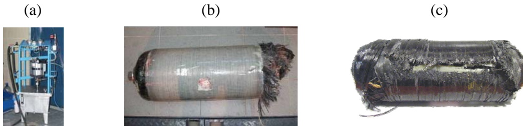
Figure 14: (a) A hydraulic burst pump, and (b,c) vessels after bursting, depending on the composite winding architecture.
