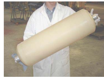
Figure 4: A PA-6 liner obtained by reactive rotomolding
