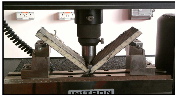
Figure 8: Three-point bending test
