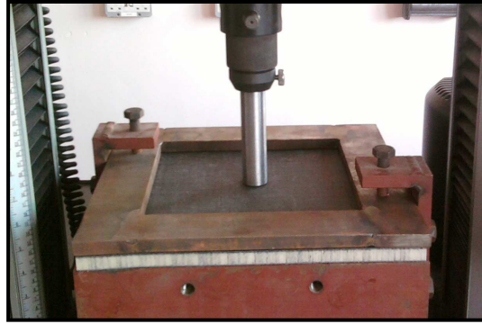
Figure 5: Quasi-static indentation test
