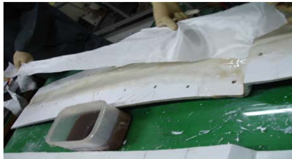
Figure 7. Lay-up process on the mold
