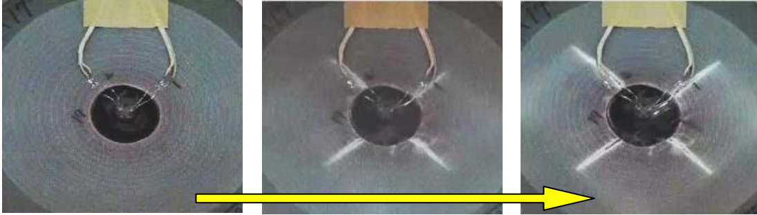
Fig.9. High Speed photograph of fracture in gauge area of cruciform specimen under biaxial loading ( F_x : F_y = 1:1 ).
