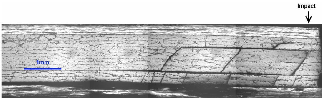
Figure 1: Impact Damage with delaminations between plies and transverse cracks on a [0_2/+60_2/-60_2]_s laminate.
