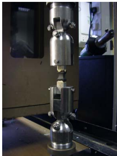
Figure 3 specimen in the jig in the tension machine
