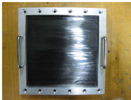
Fig. 1: Metal jig frame to dissolve resin from prepreg
