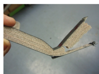
Figure 20 Experimental results of dynamic three points bending test of CF/PP and CF/EP form sandwich.
