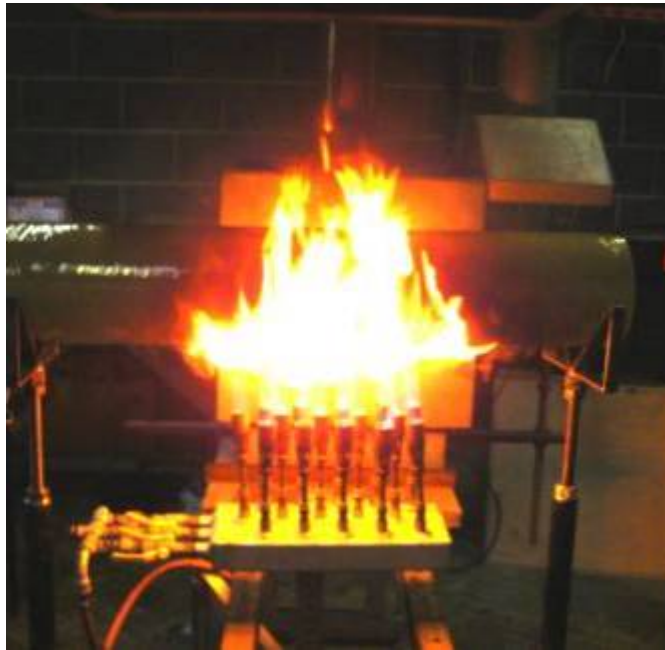
Figure 1. 200 mm diameter GRE pipe in the burner test.
