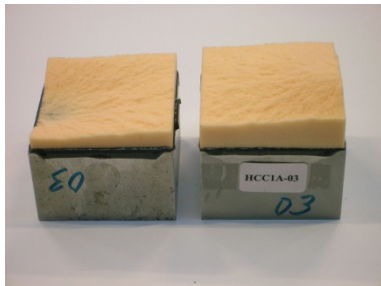
Figure 2. Test specimen, test set up, and test specimen for out-of-plane tensile testing. Extensometers are mounted to measure strain for calculation the E-modulus. failed
