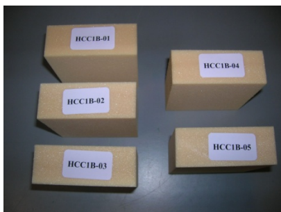
Figure 3. Test specimens and test set up for out-of-plane compression testing. The specimens is loaded in a 4 column guided pressure tool. Extensometers are mounted to measure strain for calculation the E-modulus.
