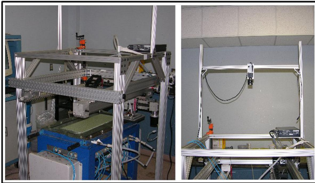
Figure 3: Left: Photograph of the workstation gantry control system and workstation. Right: Close up photograph of the camera mounted to the top of the gantry structure.
