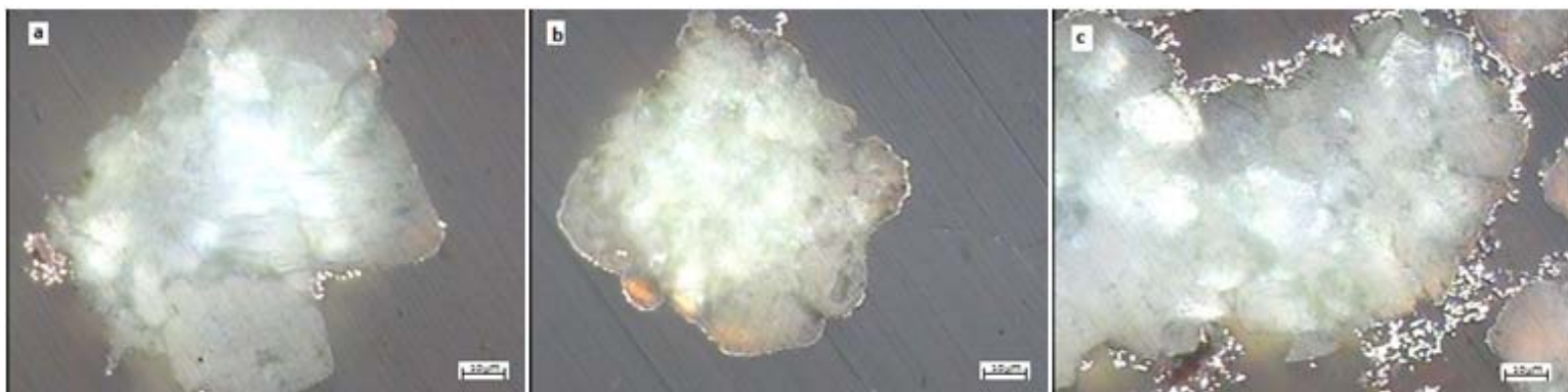
Fig. 3. OM micrograph of a) 3step activated powders, b) early stages of electroless plated powders; c) Cu coated powders at the end of plating
