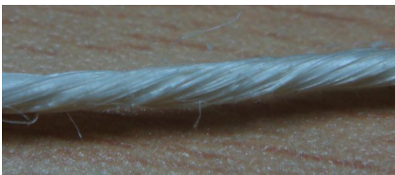
Fig 7 High level of sisal fiber yarn twist
