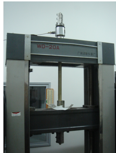
Fig. 5 tensile test of coaxial connector
