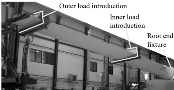
Fig. 2: The setup of the full scale test
