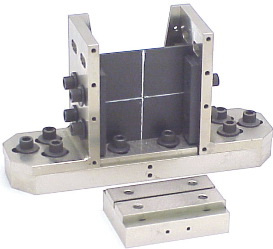
Fig. 2 Boeing fixture for CAI strength test
