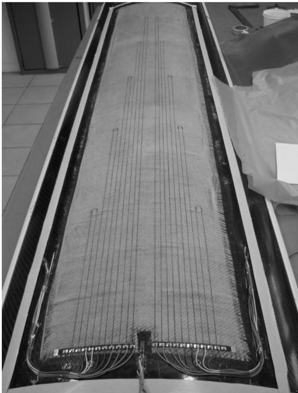
Fig.5. Underside of the CT table applied with ten, u-shaped CFS. Wiring attached to the support. CFS- Length varied from 250 - 1250 mm.
