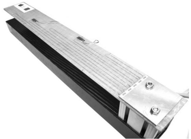
Fig.3. Small GFRP cantilever beam to verify the theoretical approach.
