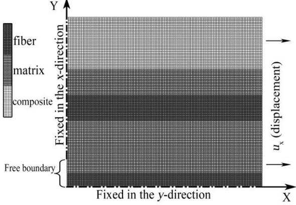
Fig.1. Finite element mesh and boundary condition.
