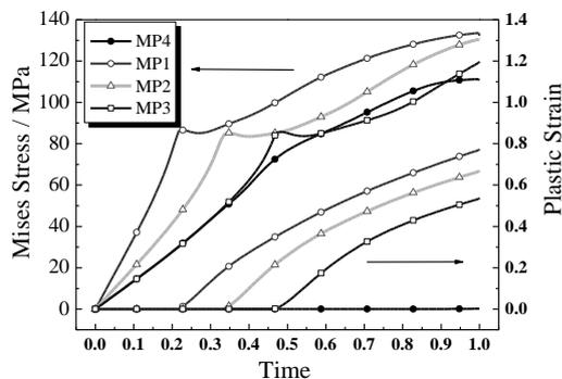
Fig. 3. Mises stress-time and accumulated plastic shear strain-time relationships for typical four Material Points (MP for short in the legend) in the composite. Note that the time represents the normalized solving process, instead of the real time.
