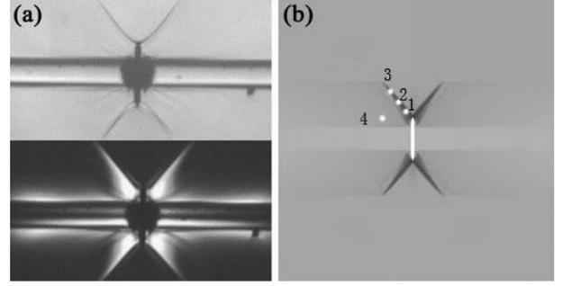
Fig. 2. Comparison between the simulated results and experimental observation. (a) optical micrograph (upside) and polarized optical micrograph (underside) of shear bands captured in our epoxy/glass fiber composite tensile test; (b) the maximum in-plane logarithmic strain contour.
