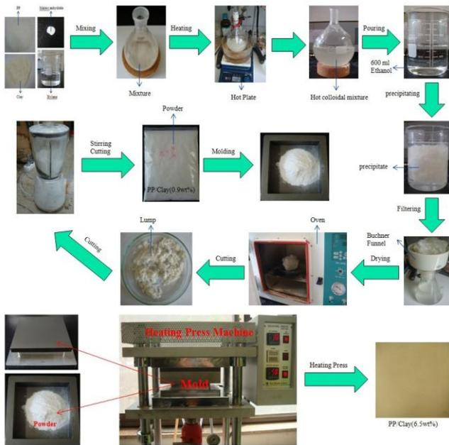
Fig. 2. Specimens fabrication process
