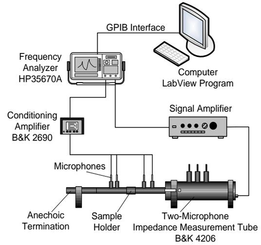
Fig. 4. Sound TL measurement system
