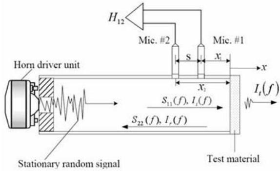
Fig. 1. Schematic of impedance tube
