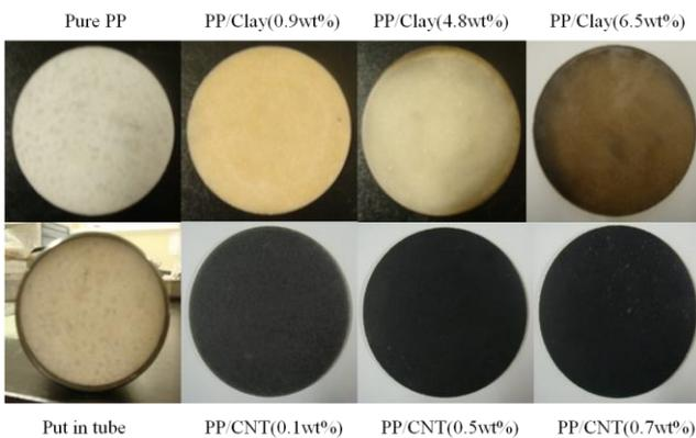
Fig. 3. PP/Clay and PP/CNT nanocomposite specimens
