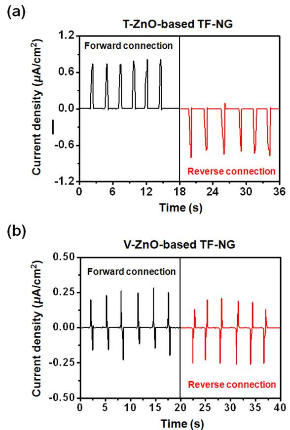
Fig.3. Piezoelectric charge generating behaviors depending on ZnO nanorod morphologies. a) T-ZnO-based TF-NG which shows DC-type charge generation. b) V-ZnO-based TF-NG that presents AC-type charge generation.
