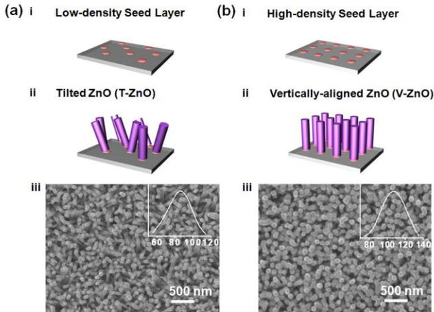
Fig.1. ZnO nanorods morphologies according to the seed density.
