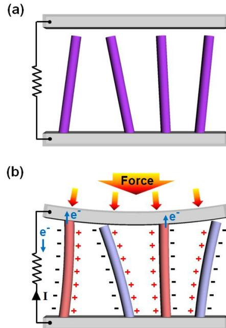
Fig.2. Schematic diagrams showing DC-type output charge generation from T-ZnO nanorods a) before and b) after application of a force.
