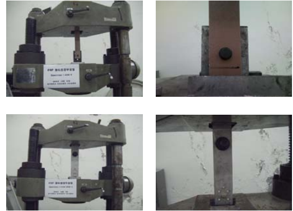
Fig. 4. Experiment of bolted connection
