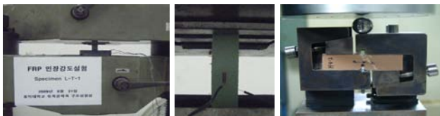
Fig. 3. Tension and shear tests
