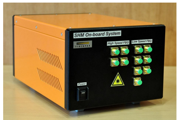
Fig.7. Prototype SHM instrument equipped with two FBG interrogators and a PZT impedance interrogator.
