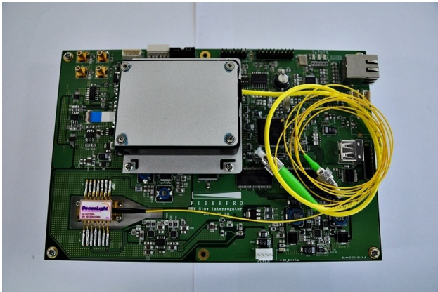
Fig.2. Printed circuit board and assembly for monitoring flight load operating at 200Hz sampling rate.
