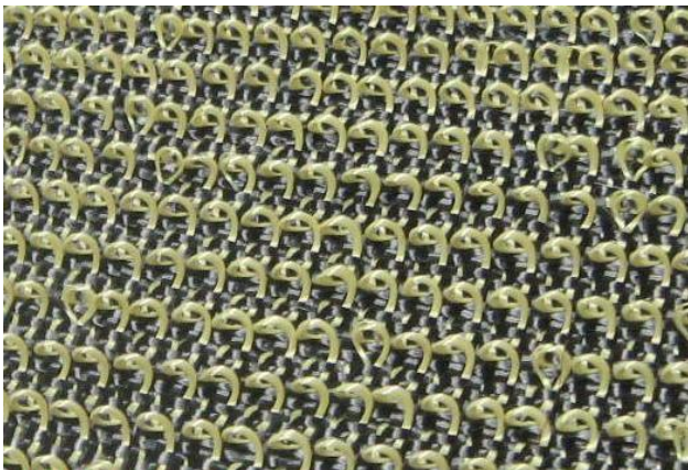
Fig.1. (2) 3D carbon fabric (Base 2D fabric is carbon fiber, hook and loop are aramid fibers). Width: Min./ Max. 0.4/1.80m Unit Weight: 100-600g/m 2 Yarn Diameter: 3-12K/800-3000D
