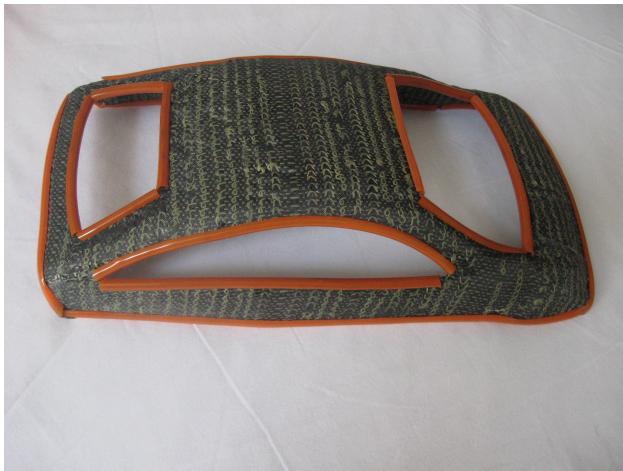
Fig. 3. A car body model is made by the partially automatic lay-up fabric method and RTM process.
