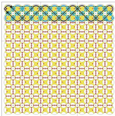
Fig. 2. 3D braiding pattern utilized for the rectangular cross section preform fabrication.
