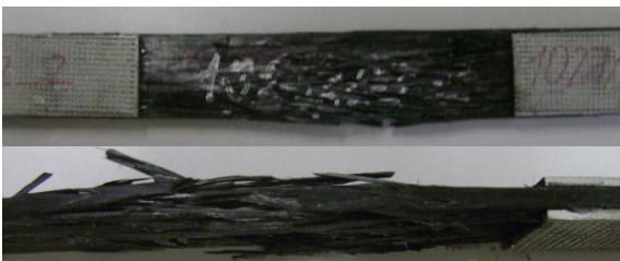
Fig. 4. Fatigue failure of a specimen.
