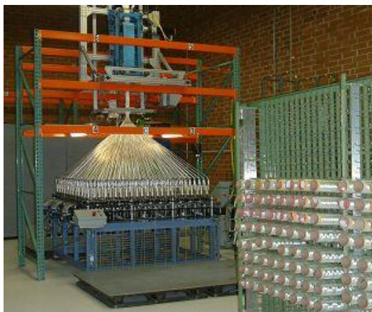
Fig. 1. 3D rotary braiding machine at 3TEX, Inc. with full 576-carrier fiber set up and axial fiber supply from the creel.
