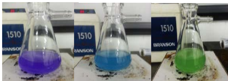
Figure 2: Change in Color indicating reaction endpoint.
