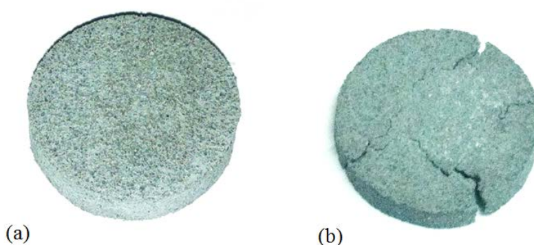
Figure 10: The PBX samples recovered. (a) The strain rate 1292 \text{ s}^{-1} ; (b) the strain rate 2000 \text{ s}^{-1}
