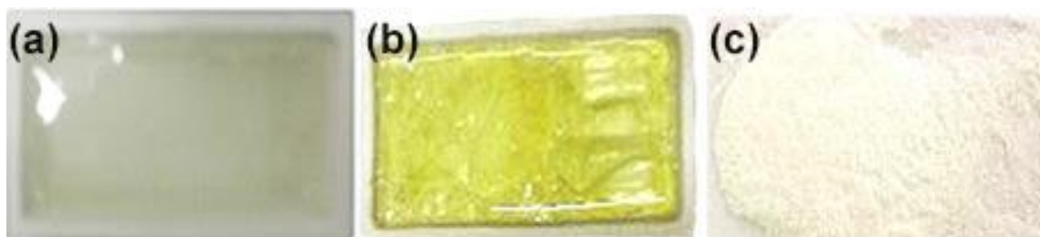
Figure 1: Macroscopic photo of the samples (a) the liquid SiCN precursor; (b) curing precursor; (c) precursor powders.
