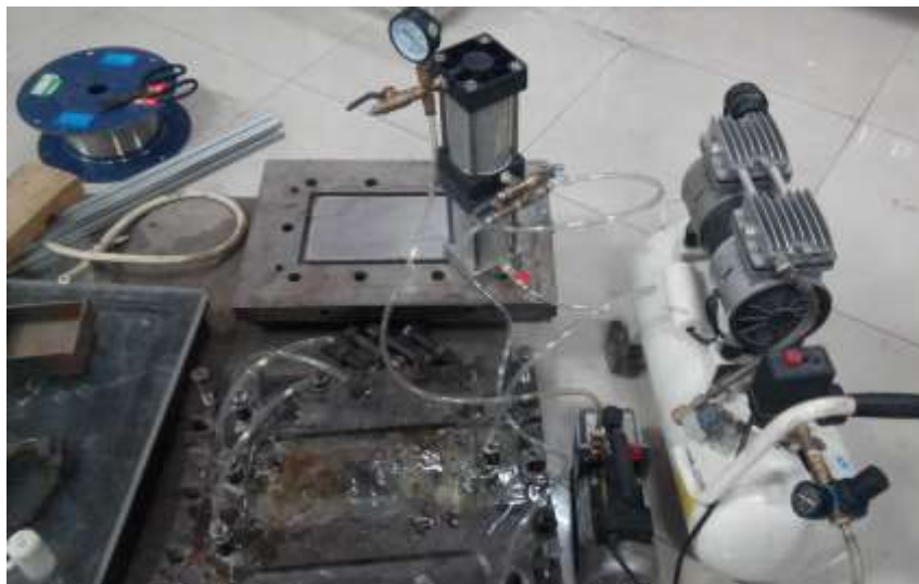
Figure 3: Schematic for preparation of CF/EP composites.
