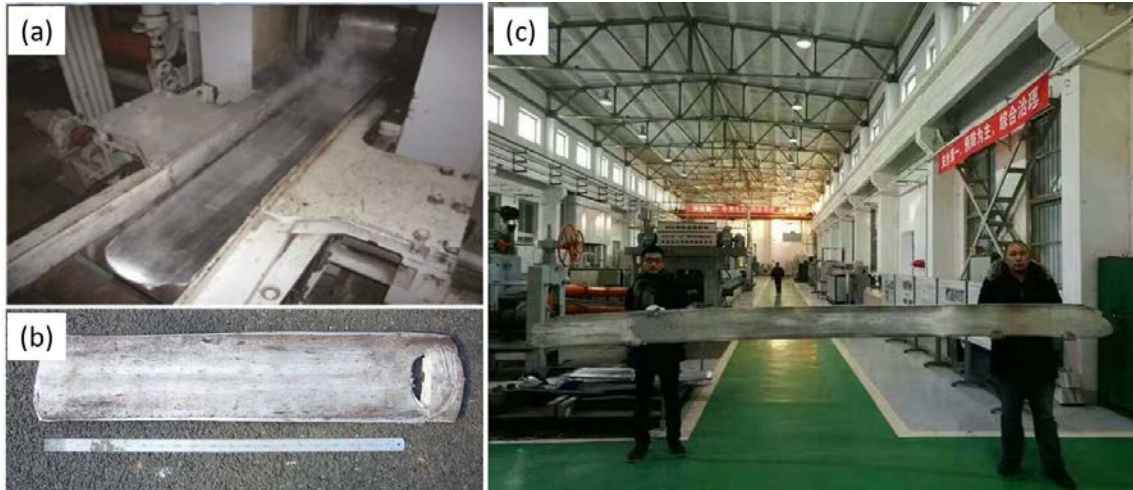
Fig.2 (a) The hot rolling process and BRALC plates with thickness of 20mm (b) and 3mm (c)
