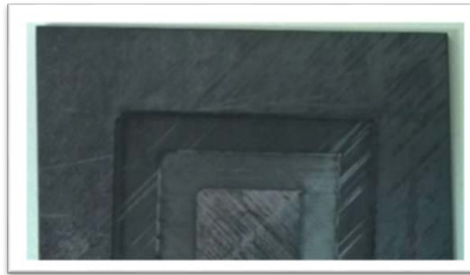
Figure 2: An example of step scarfing on a composite sample
