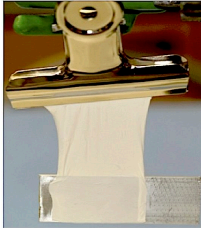
Figure 3: Modified PTFE sheet glued to an Al-board with PVP glue.
