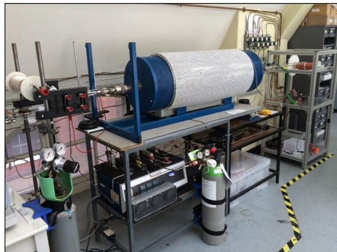
Figure 2. Photograph of the continuous CVD line set-up.
