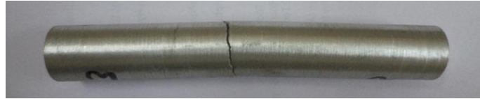
Figure 6: Flexural test specimen
