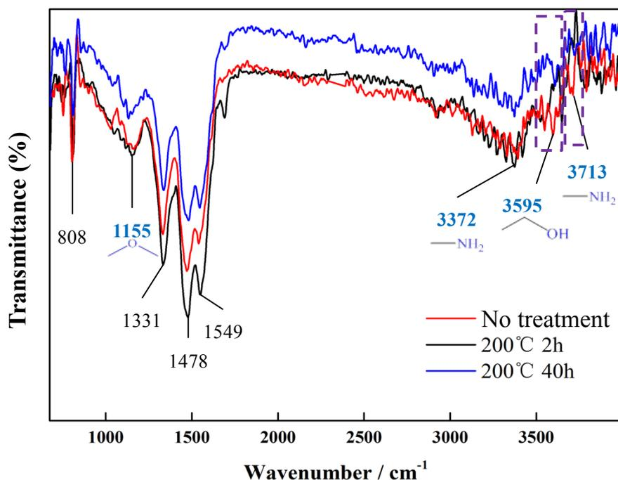
Fig 4. FRIT spectra of MF with/without thermal treatment
