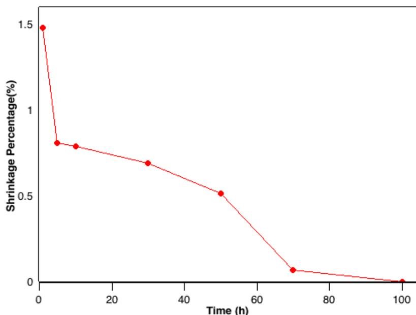
Fig 2. Relationship of time and Shrinkage percentage while thermal treating
