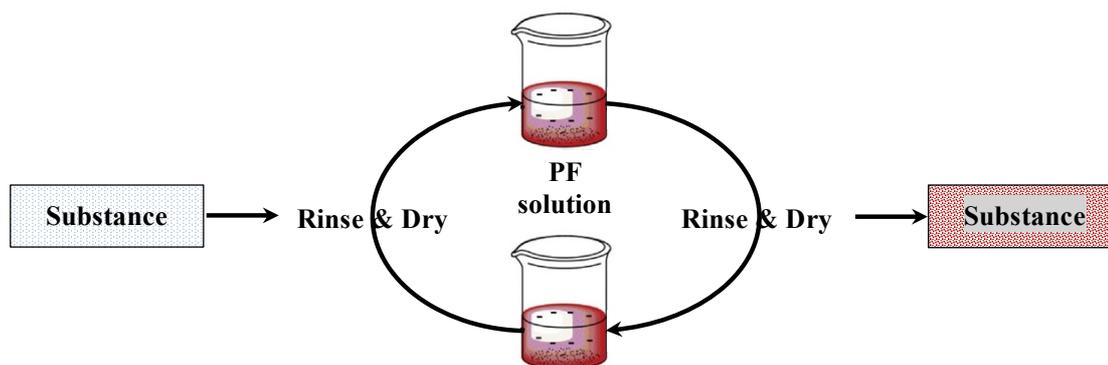
Fig 1. Schematic representation of layer-by-layer (LbL) assembly with PF solution. This process was repeated until the desired number of bilayers were deposited.
