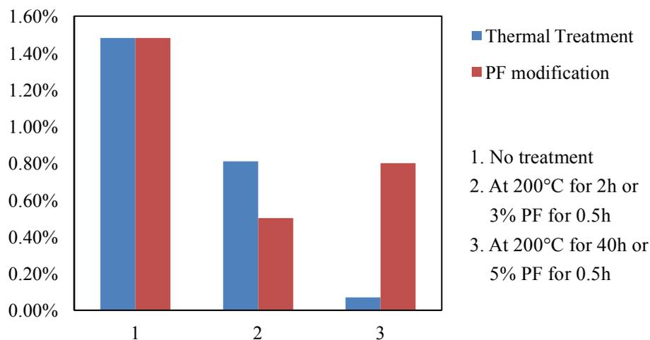
Fig 3. Shrinkage resistance of MF with different treatments
