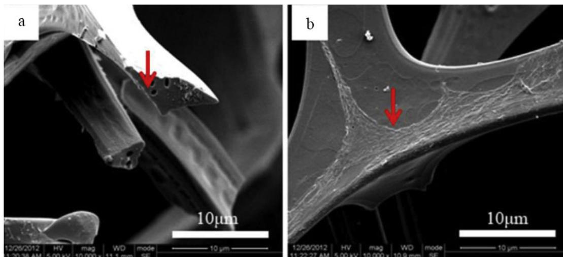
Fig 6. SEM of PF coating on MF
