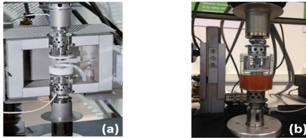
Figure 1 Metravib DMA+ 450 viscoanalyser equipped with thermal flux tool: (a) cell for V= 5\text{mL} and (b) Cell for volume up to 50 mL.
