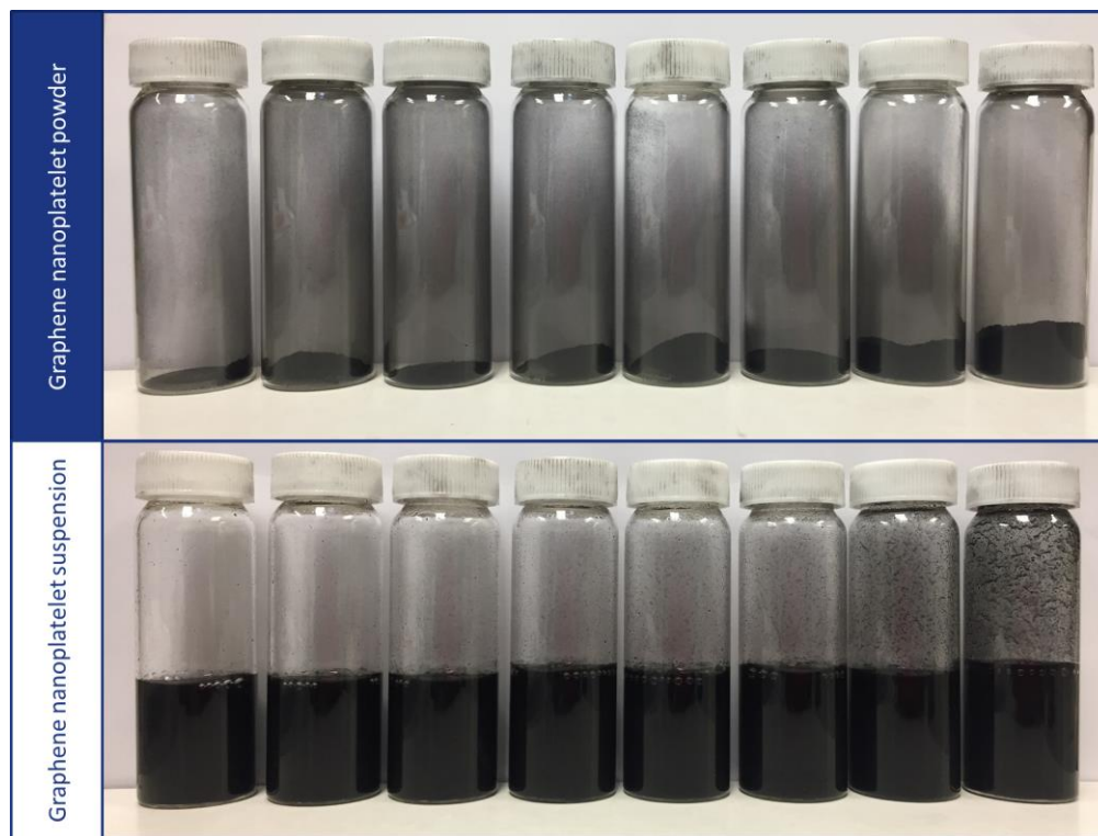
Figure 1. Top: Graphene nanoplatelet powders. Bottom: Resorcinol/formaldehyde/water with graphene nanoplatelets in suspension at loadings of, from left to right, 0.2, 0.4, 0.8, 1.2, 1.6, 2.0, 4.0, 7.5 wt.% (after bath sonication).
