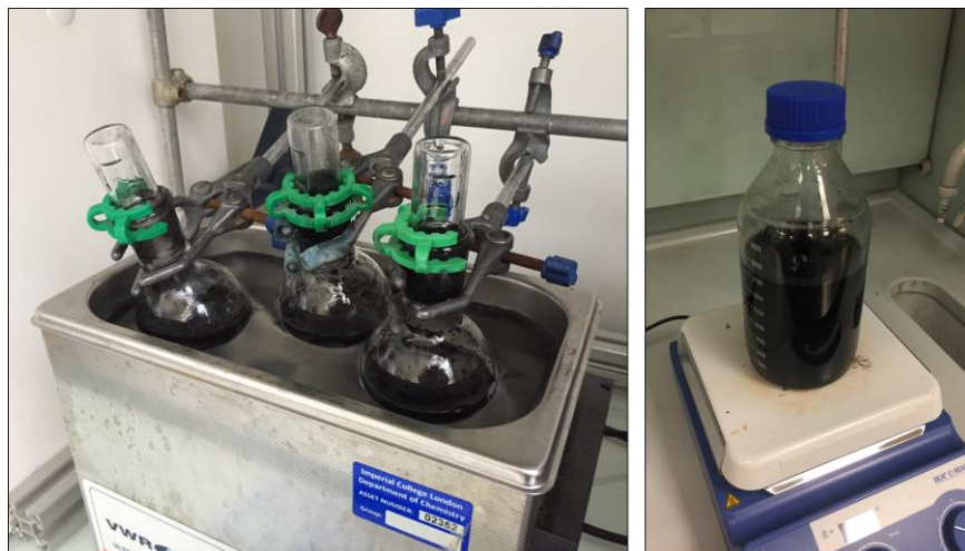
Figure 3. Left: Photograph of suspension of formaldehyde, water and graphene platelets sonicating. Right: Photograph of modified carbon aerogel precursor suspension stirring before infusion.
