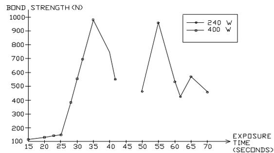
**Figure 6: Bond Strength of Nylon 66/GF (33%) with Araldite Using FFM**
