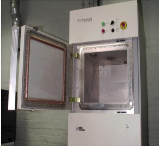
**Figure 1: Cavity of Microcure 2100 Model 250 with Frequency Range of 2 - 7 GHz and a Maximum Power of 250 W**
