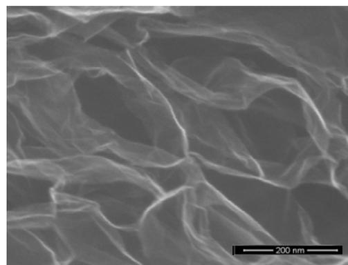
Fig. 1. SEM image of the Graphene
