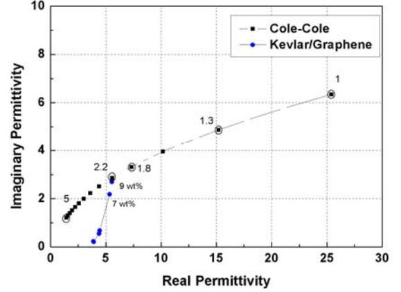
Fig. 6. Cole-Cole plot and Kevlar/Graphene/epoxy composites permittivity at 15 GHz
