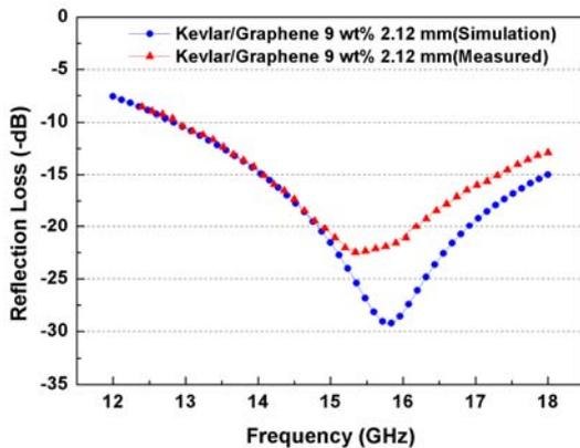
Fig. 9. Simulation and measured value of Kevlar/Graphene/Epoxy composite
