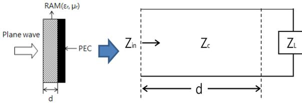
Fig. 5. Schematic design of single layer absorber (left) and transmission line equivalent circuit (right)
