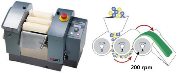
Fig. 2. Three-roll-mill and rotating speed
