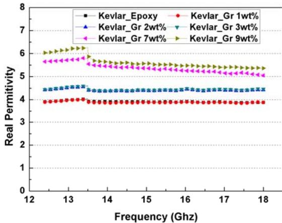
Fig. 3. Real permittivity of Kelvar/Graphene/epoxy composites
