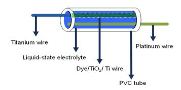
Fig. 1 A schematic of the fibrous flexible DSSC based on metal wire
