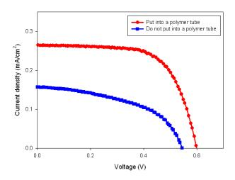
Fig. 6 I-V curves of the DSSCs fabricated with  $Zylon^{\circledast}$
