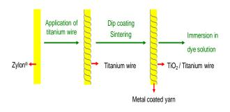
Fig. 2 A schematic of the cell applied  $\operatorname{Zylon}^{\mathbb{B}}$  as an electrode
