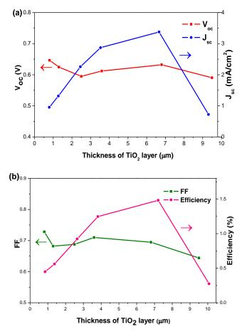
Fig. 5 Photovoltaic characteristics of fibrous DSSCs fabricated with various thickness of  $TiO_2$  film; (a)  $V_{oc}$  and  $J_{sc}$  and (b) FF and Efficiency
