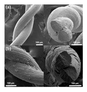
Fig. 3 SEM images of Ti wire coated with various  $TiO_2$  film thicknesses; (a)  $TiO_2$  layer thickness - 0.8  $\mu$ m and (b)  $TiO_2$  layer thickness - 9.5  $\mu$ m.
