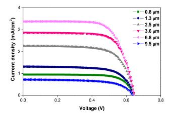
Fig. 4 I-V curves of fibrous DSSCs fabricated with various thickness of  $TiO_2$  film
